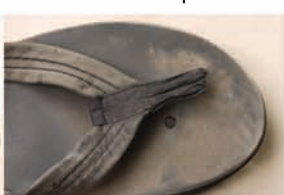
Torn toe straps
